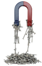
Magnetic force can act over a distance to attract the iron nails.
